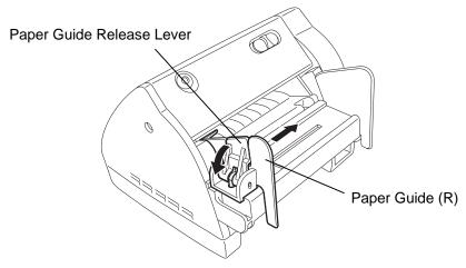
**3.** Remove the two screws to detach the Paper Guide Unit from the printer.
